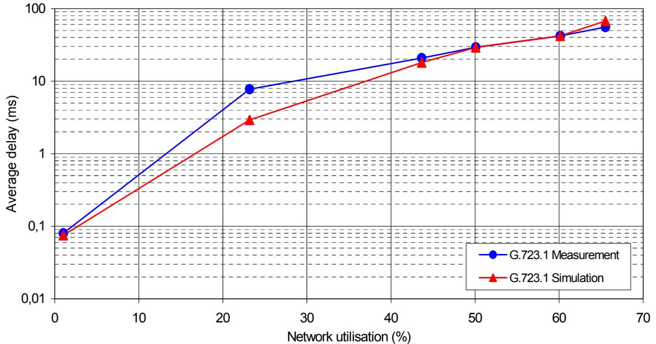
Figure 2: Comparison of delays on a loaded network between PC telephones and simulation results
