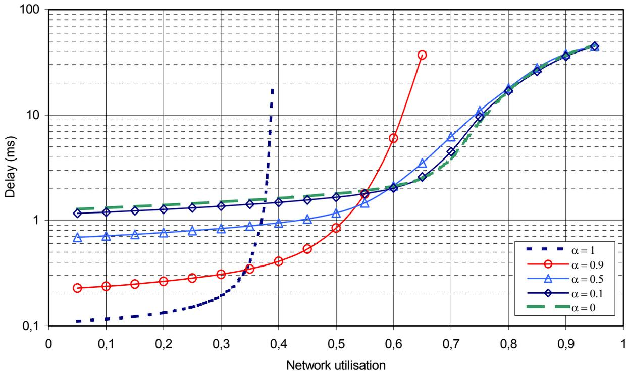
Figure 1: Average delay with regards to network utilisation and the proportion of short frames ( $\alpha$ )
