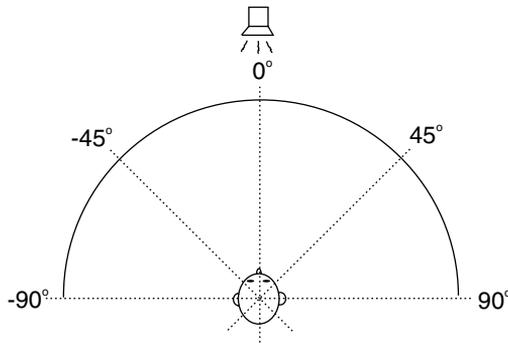
Fig. 6. The central position used to measure directional resolution.
