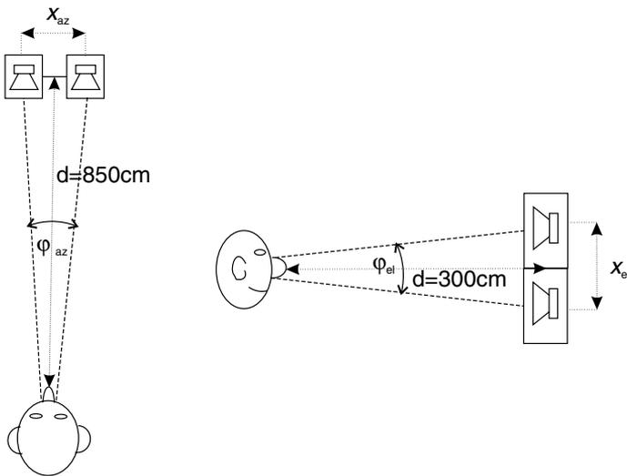
Fig. 7. Loudspeaker set-up for azimuth and elevation resolution measurements.
