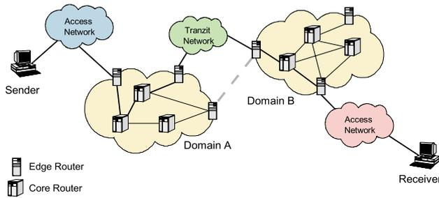
Fig. 1. Referential DIS network topology
