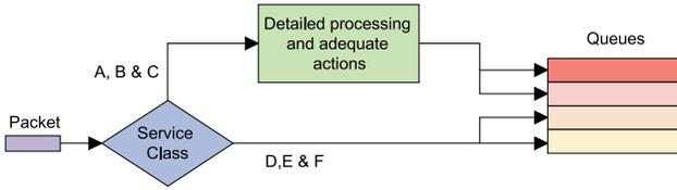
Fig. 2. A simplified packet processing flow in a proposed DIS network
