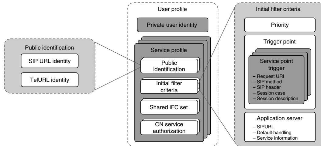
**Fig. 6** User and service profiles. User profiles represent a collection of services data and user-related data, i.e., user identities and service profiles (subscribed services, their configuration, personalization information, etc.).
