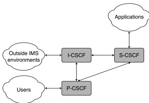
**Fig. 3** CSCF. In IP IMS, three functionally different implementations occur. S-CSCF provides control functionalities for user authentication, session routing, and service control. P-CSCF represents the first point of contact in IMS from user side, while I-CSCF represents the first point of contact from other IMS environments.
