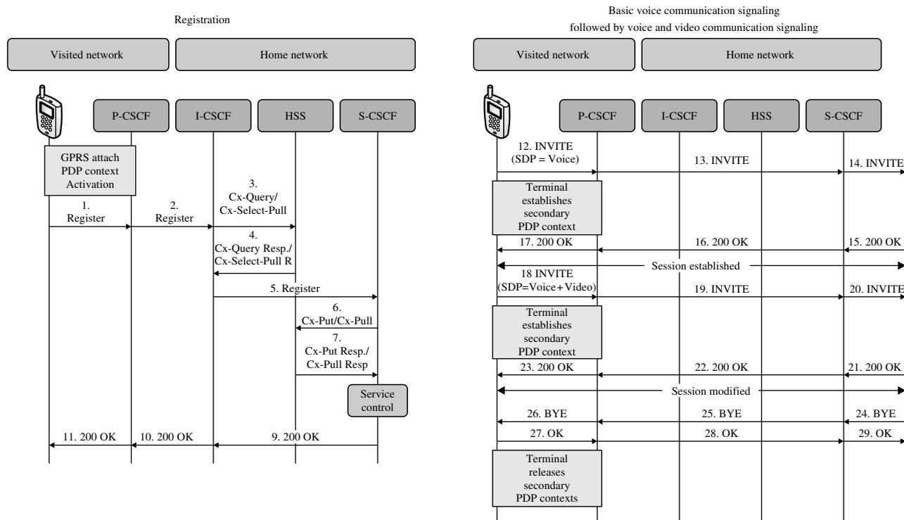
Fig. 8 Registration and basic communication of an IP IMS user with indicated IP-CAN establishment for gateway GPRS/UMTS. Message flow is SIP-based, procedures involve basic IMS entities, PDP context activation events are indicated.
