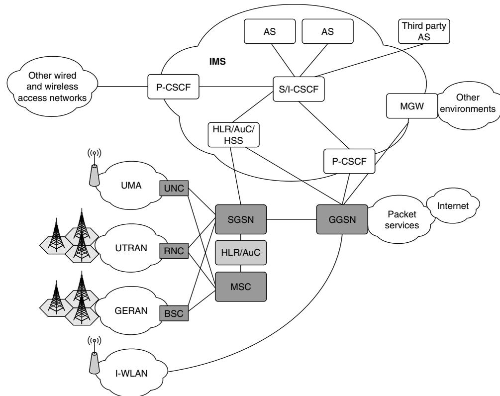
**Fig. 9** A detailed schema of introducing IP IMS into mobile system. Existing circuit-switched (GERAN/UTRAN, and MSC as a core entity) and packet-switched [GERAN/UTRAN access network and service GPRS support node (SGSN) and gateway GPRS support node (GGSN) as core entities] segments are retained while IMS segment is introduced in parallel. Most common mobile solution exploits existing packet-switched segment to access IMS and its services.
