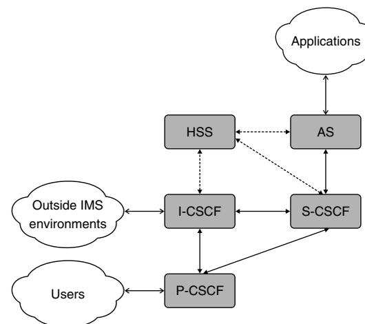
**Fig. 7** Basic IP IMS entities. While AS provides service logic invocation and execution, S-CSCF is engaged in routing and service control based on user and service information, stored in HSS. P-CSCF and I-CSCF provide access functionalities.
