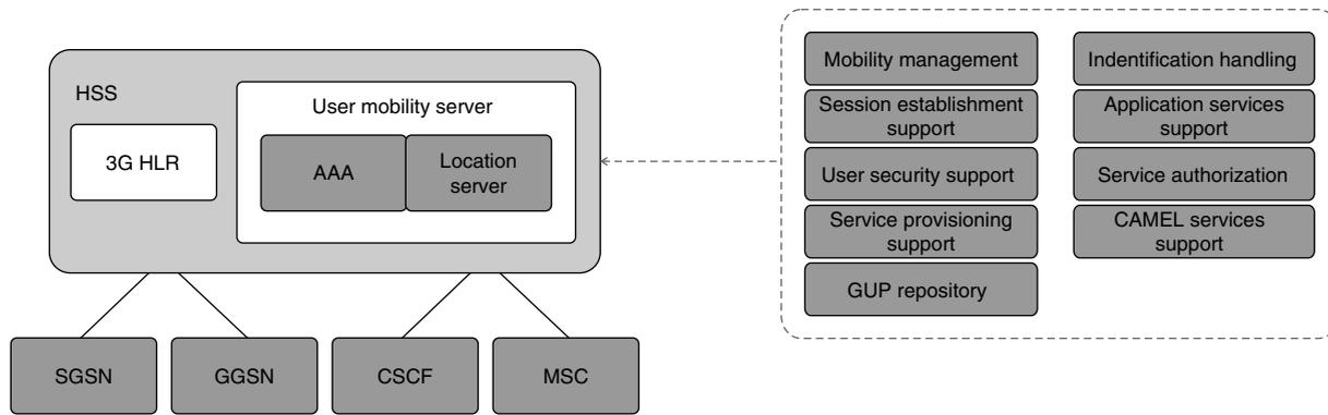
**Fig. 5** Generic HSS structure, basic interconnections, and capabilities. HSS serves to support session control and management and is a shared entity for all subsystems inside heterogeneous communications environment, e.g., circuit-switched, packet-switched, and IP IMS domain of a migrated 3G mobile system.
