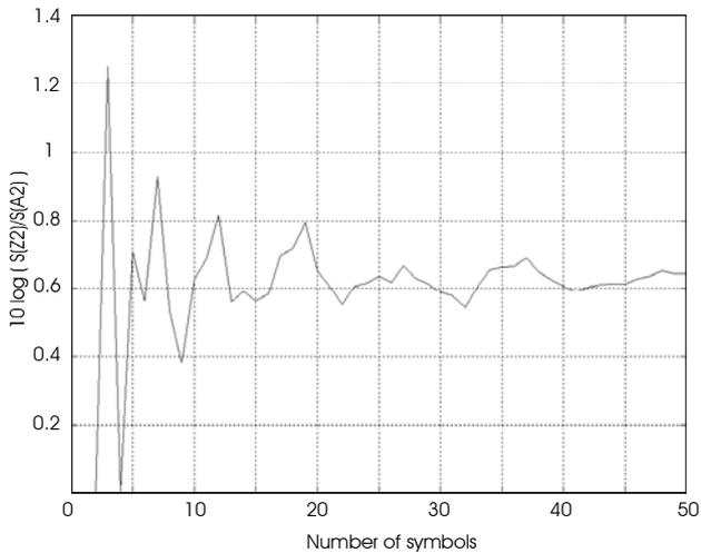
Figure 4: Coding gain of  $A_2$  lattice with small number of symbols
