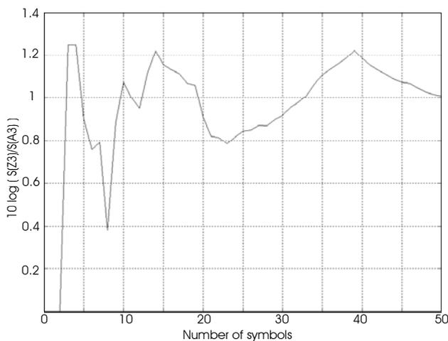
Figure 5: Coding gain of  $A_3$  lattice with small number of symbols
