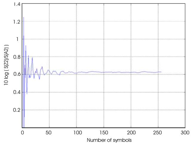
Figure 2:  $A_2$  lattice coding gain dependence on the number of symbols
