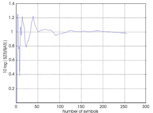
Figure 3:  $A_3$  lattice coding gain dependence on the number of symbols
