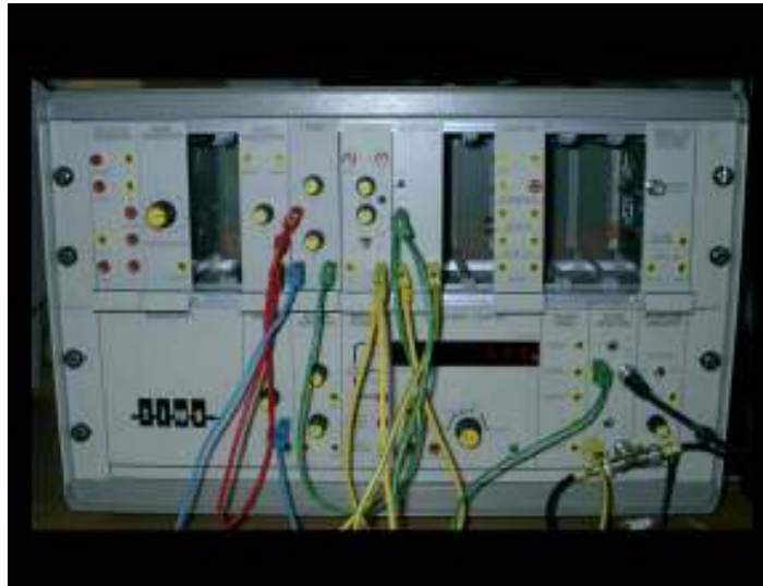
Zgled : AM-DSB-LC modulator z moduli TIMS
